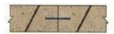
BUILT-IN BUILDING JOINT PVC WATERSTOP
