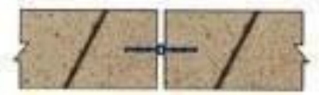
BUILT-IN EXPANSION JOINT PVC WATERSTOP
