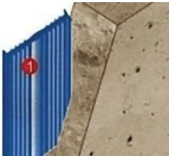
INTERNAL CONSTRUCTION JOINT PVC WATERSTOP
